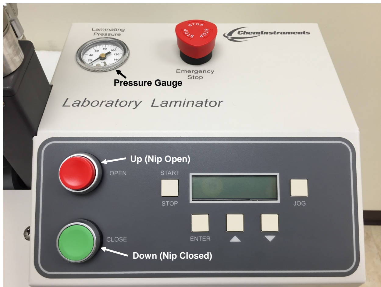
Photo 4 - Control Cabinet Front Panel
